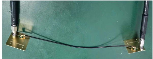
NRF215 Jump wire (OD.1.13 cable, L=10cm ), Mating with two test PCB sets ( Included Two 2.92BM Connectors )
